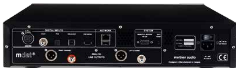
ABOVE: One of every digital 'flavour' is offered here – AES/EBU, coaxial, optical, USB-B for computer connection, USB-A for an external drive/device, and wired Ethernet. Analogue outputs are offered on balanced XLRs and single-ended RCAs
