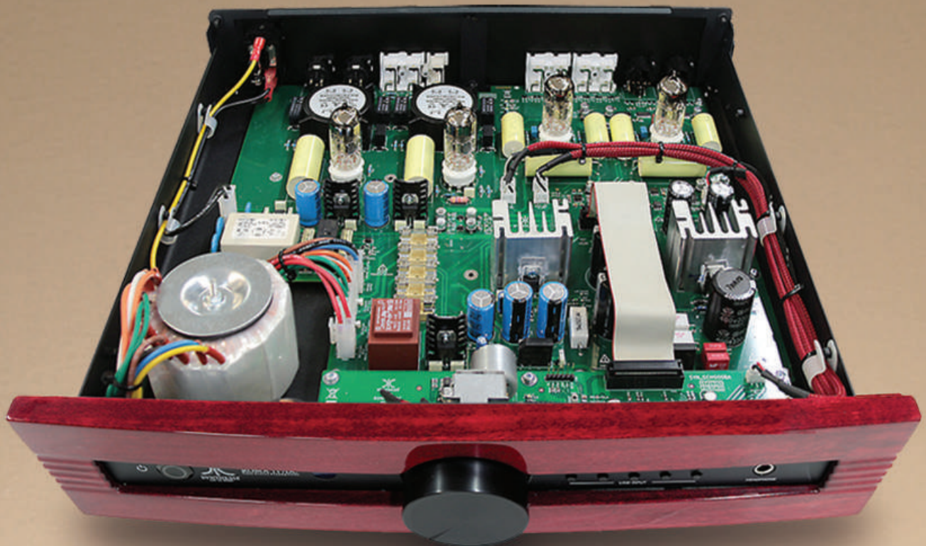
Internal view: Clean, mechanically stable Output transformer, ALPS potentiometer.
